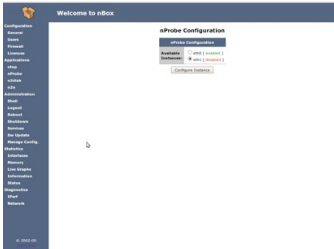
Fig. 6 – nBox: nProbe Configuration Page, selection of the network interface.
