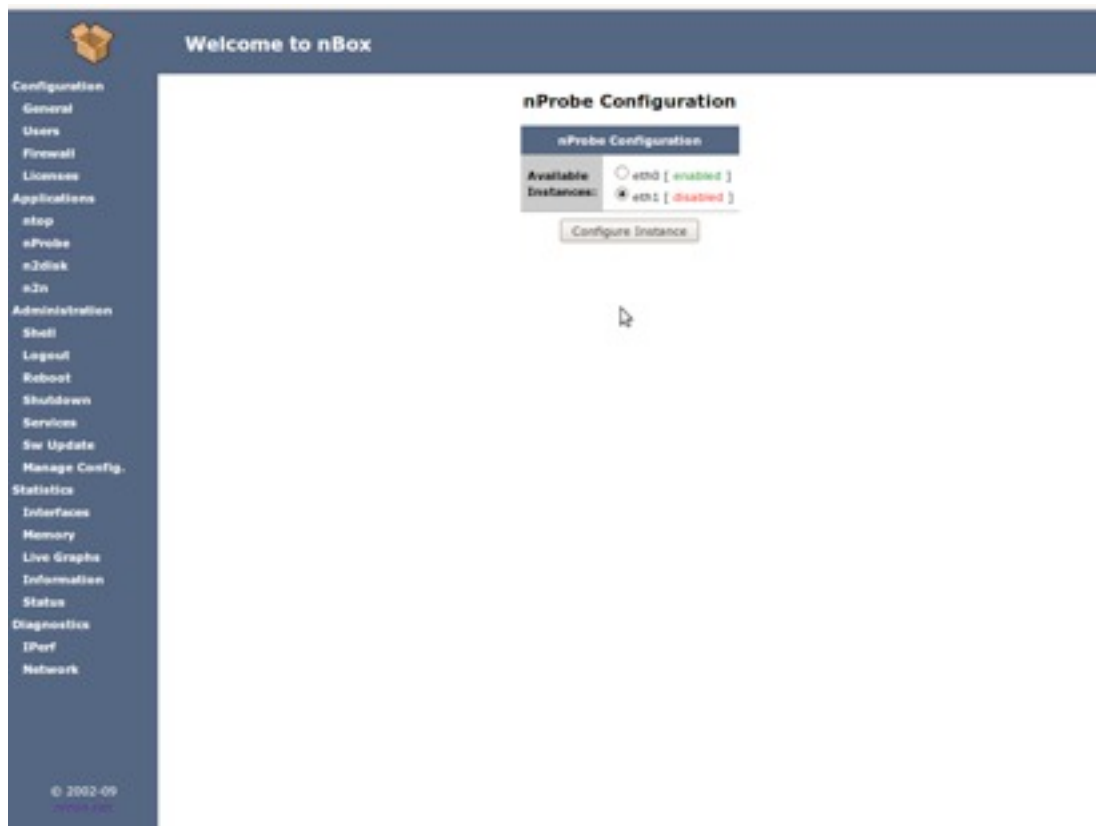
Fig. 7 – nBox: nProbe Configuration Page for the selected network interface.
